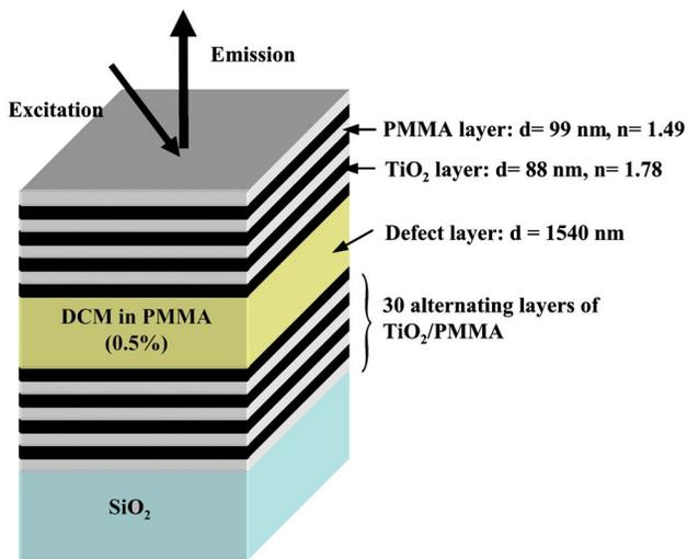
FIG. 1. (Color online) Schematic of dye-doped defect-mode 1-D photonic crystal, glass-(PMMA-TiO<sub>2</sub>)<sup>15</sup>-(DCM/PMMA)-(TiO<sub>2</sub>-PMMA)<sup>15</sup>-air.
