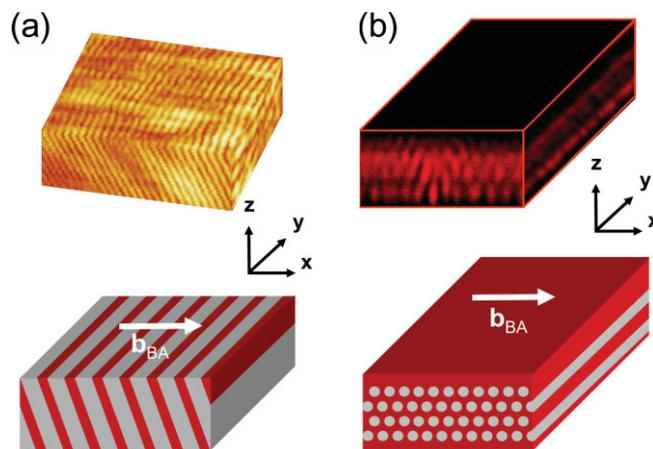
**Figure 2.** 3D reconstruction of reflection-mode LSCM images of highly ordered a) lamellar and b) cylindrical PS- $b$ -PI BCPs in thin films obtained from the DS process. 3D imaging revealed that lamellae were tilted by about 60° to the fast-growth direction of BA and cylindrical microdomains were hexagonally packed in the  $xz$ -plane. Corresponding schematics with the direction of BA crystallization are also shown.
