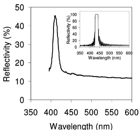
**Figure 2.** Experimental reflectivity spectrum of the fabricated block-copolymer-based distributed Bragg reflector at near-normal incidence using a reflection-mode optical microscope connected to a fiber-optic spectrometer. The inset shows a calculated reflectivity spectrum using the transfer matrix method at a normal incidence for a finite 1D periodic structure, assuming 300 layers of PS (76 nm,  $n = 1.59$ ) and PI domains (64 nm,  $n = 1.51$ ).
