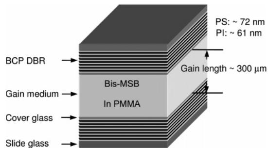
**Figure 4.** Schematic of the block-copolymer-based laser cavity, composed of a gain medium, Bis-MSB and PMMA, enclosed between two block-copolymer-based distributed Bragg reflectors. The thicknesses of PS and PI domains are estimated values at 10 wt % solvent concentration based on the peak position and fwhm of the reflectivity spectrum.<sup>19</sup>
