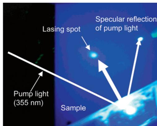
**Figure 6.** Photograph of the 410 nm lasing from the block-copolymer-based laser structure. A highly directional lasing output in the backward direction was observed on a white background.
