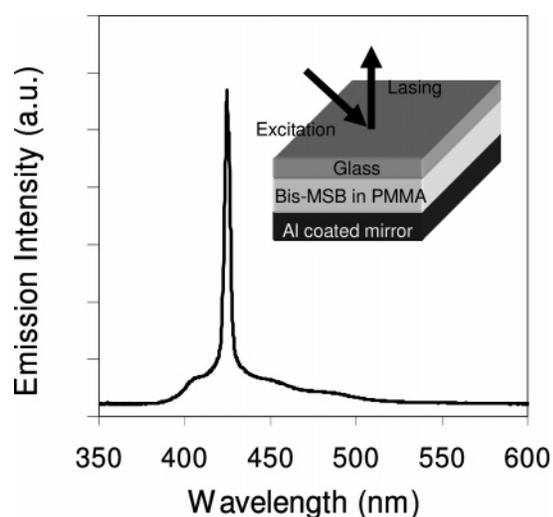
**Figure 8.** Lasing spectrum from a solid film of Bis-MSB (0.1 wt %) in PMMA sandwiched between an aluminum-coated mirror and a glass slide pumped by a 355 nm pulse laser, where the lasing peak occurs at 425 nm and the FWHM is 4 nm. The inset shows a schematic of the sample.
