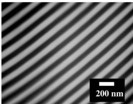
**Figure 1.** Bright-field TEM micrograph of cryomicrotomed PS-*b*-PI block copolymer showing a 1D periodic lamellar morphology, in which the dark regions correspond to PI domains preferentially stained with OsO<sub>4</sub> and the bright regions correspond to PS domains. The domain periodicity is approximately 140 nm (PS, 76 nm; PI, 64 nm).
