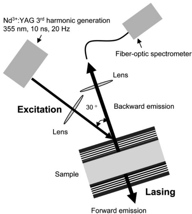
**Figure 5.** Schematic of the experimental setup for measuring the lasing output from the BCP/gain/BCP device.
