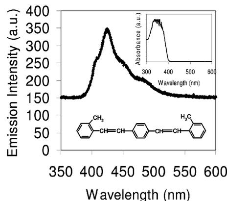
**Figure 3.** Photoluminescence (PL) spectrum from a solid film of Bis-MSB (0.1 wt %, 355 nm excitation) in PMMA. The fwhm of the PL spectrum is about 41 nm. The inset shows the absorption spectrum from the same sample, where the absorption maximum is located at around 350 nm.
