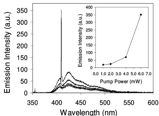
**Figure 7.** Emission spectra obtained at various pump powers. The fwhm of the lasing peak is 1 nm. The inset shows the emission intensity at the lasing wavelength (410 nm) as a function of pump power, which clearly shows a threshold for lasing at around 4 mW pump power (0.2 mJ pulse energy).
