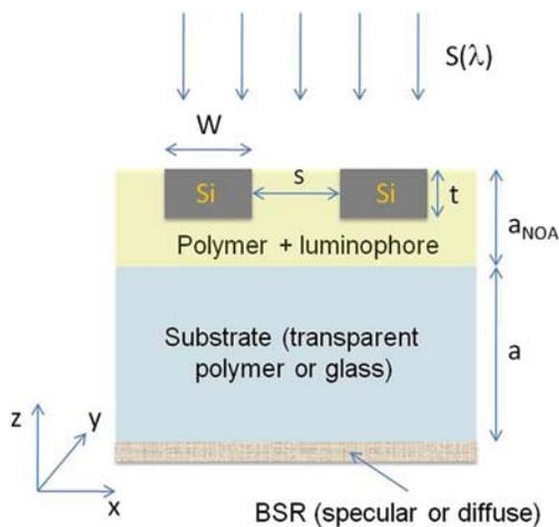
Fig. 1. (Color online) Cross section of the solar concentrator for ultrathin Si microcells.
