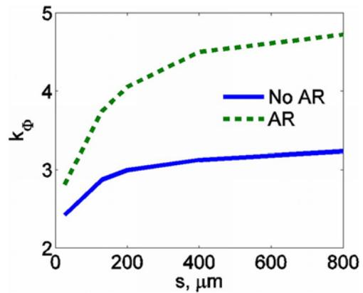
Fig. 7. (Color online) Indirect gain of a microcell array with and without ideal AR surfaces as a function of separation between microcells,  $W = 50 \mu\text{m}$ ,  $a = 1000 \mu\text{m}$ , glass substrate, luminescent solar concentrator, specular reflector, and  $R_0 = 0.98$ .
