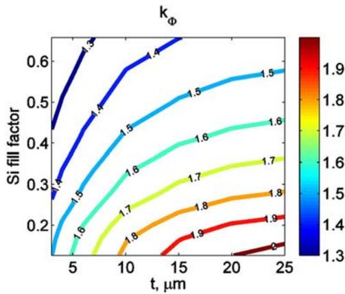
Fig. 5. (Color online) Indirect gain of a Si microcell array with a nonluminescent concentrator as a function of the microcell fill factor and microcell thickness.  $W = 50 \mu\text{m}$ ,  $a = 1000 \mu\text{m}$ , glass substrate, ideal Lambertian reflector.
