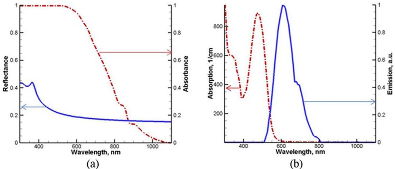
Fig. 2. (Color online) Optical properties. (a) Si normal reflectance in NOA and  $15\ \mu\text{m}$  Si slab normalized absorbance, Si properties from [13], (b) absorption and emission spectra for DCM.
