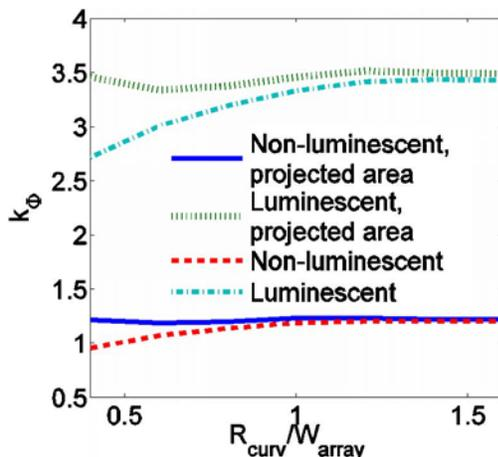
Fig. 6. (Color online) Indirect gain of a deformed Si microcell array,  $W = 50 \mu\text{m}$ ,  $s = 100 \mu\text{m}$ ,  $a = 30 \mu\text{m}$  with luminescent and nonluminescent concentrators, specular reflector,  $R = 0.98$ , as a function of the bending radius normalized to the width of substrate. Curves labeled “projected area” show indirect gains calculated with the normalization to a flat system with the same projected area.
